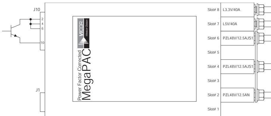
Figure 6. Enable/Disable Control of Maxi Arrays
